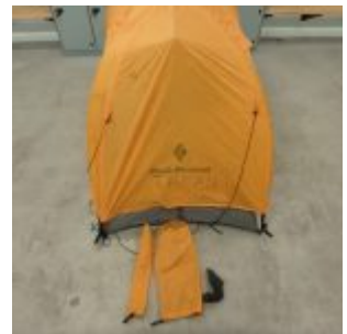
Black Diamond Tent M01 – Repaired outer; delaminating outer
