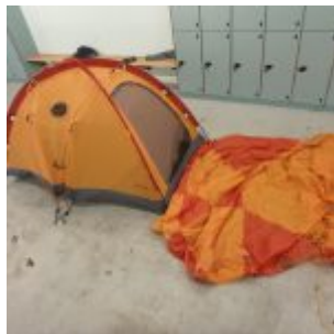
Marmot Asgard 2P A4 – Delaminating Outer; a pole had been repaired
